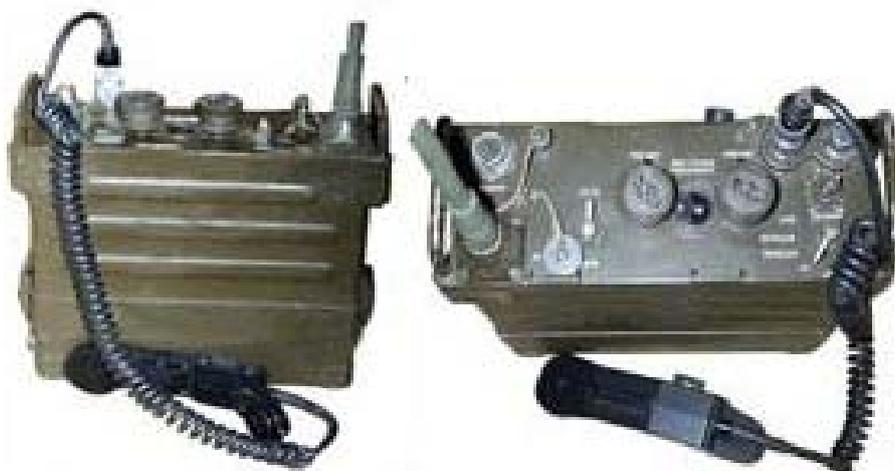
The AN/PRC-25 Radio weighed 23.5 lbs (10.6 kg), heavier than the GPMG M60. It was however a very robust piece of equipment which was virtually shock proof as well as being water proof.
